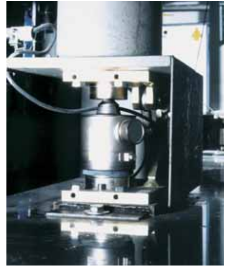
Tank and vessel weighing
