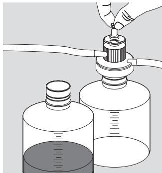
Place Sartolab® 150v on the bottle neck. A vacuum is automatically created when used with a water jet pump or other vacuum source.
