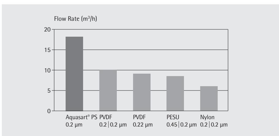
30" Filter cartridges at 1 bar | 14.5 psi differential pressure (20°C)
