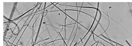
Loose glass microfibers under a microscope
