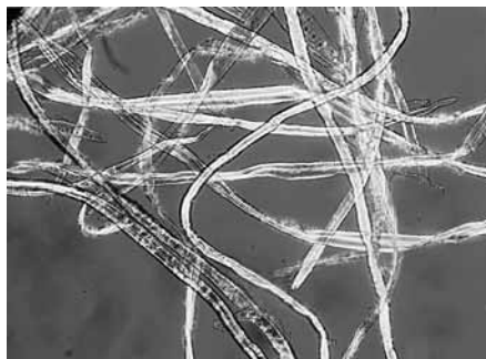
Non-bound cellulose fibers under a microscope
