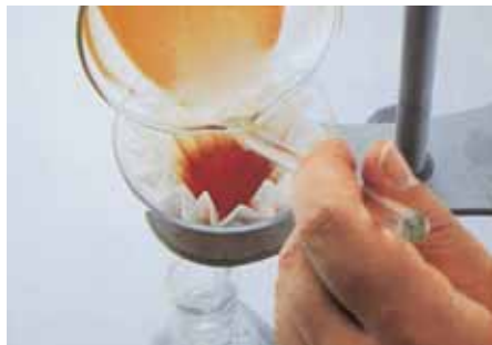
Filtration using a folded filter in an analytical funnel
