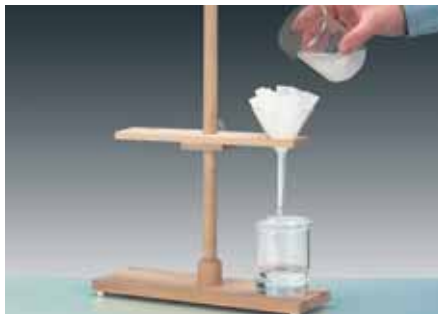
Completely folded filter Courtesy of Phywe Systeme GmbH
